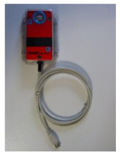
At the Download Station, there will be a Master Station attached to a computer which will read your finger stick. You simply put your finger stick in the hole of the Master station until it beeps, then remove it. Follow instructions given by the computer operator. You will receive a paper slip showing your elapsed time and your splits at each control. If there is a problem with your Results, go to the complaint taker to straighten it out.
